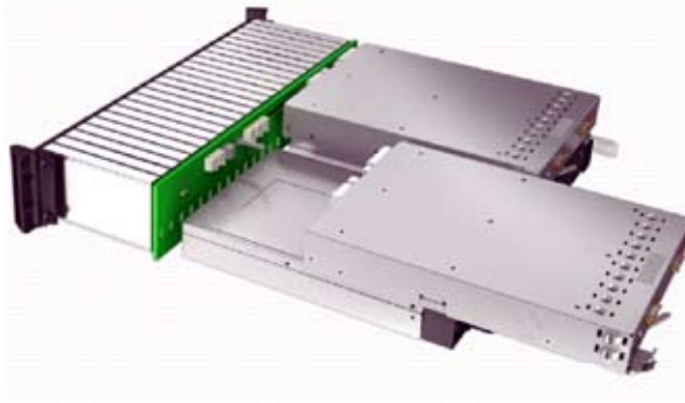
Figure 1: Dual-redundant storage server
